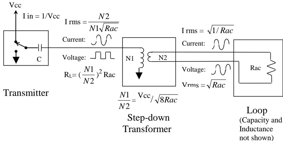
Figure 1: Block diagram of major components including Signal computations for a 1W system
