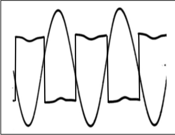
Figure 2 Scope waveforms for base drive balance adjustment. (The square wave is the waveform at the transistor collector junction and the sine wave is the current in the loop)
